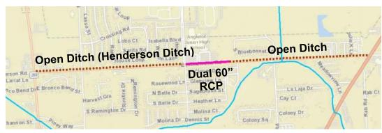
Figure 2. Existing Drainage System
