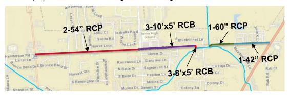
Figure 3. Proposed Storm Sewer System
