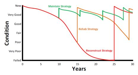
Figure 1. Pavement Life Cycle Curve
