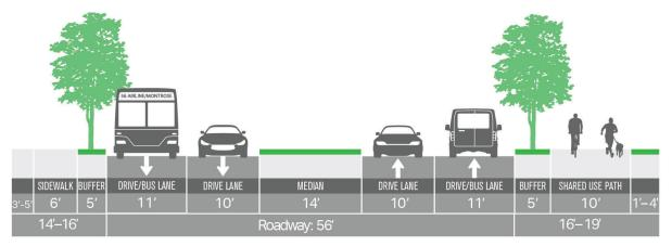
Figure 4 – Recommended Typical Section: W Dallas Street to Allen Parkway
