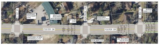
Figure 19 Foster Drive Proposed Schematic between S 1st St and S 3rd St
