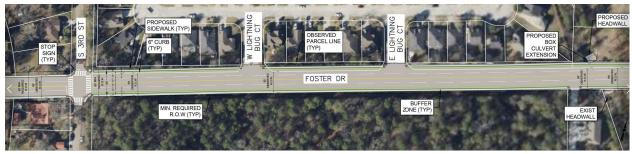
Figure 21 Foster Drive Proposed Schematic between S 3rd St to the Wetland
