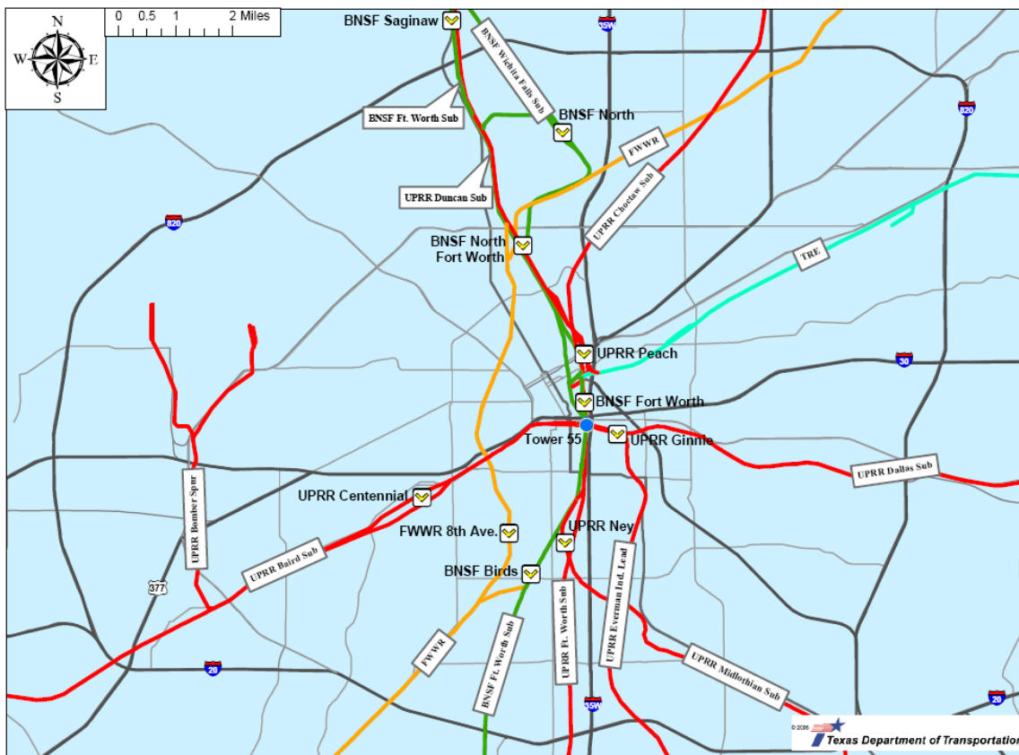
Figure 3-10: Existing Rail Network in Downtown Fort Worth (Tower 55)
