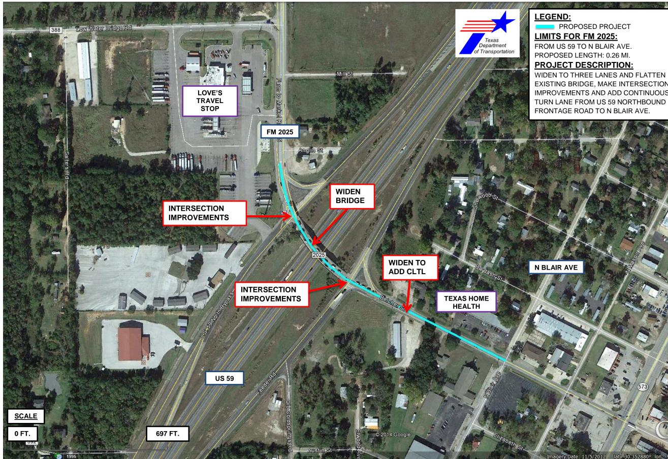
PROPOSED PROJECT WIDEN TO THREE LANES AND FLATTEN EXISTING BRIDGE, MAKE INTERSECTION IMPROVEMENTS AND ADD CONTINUOUS LEFT
