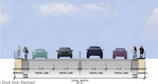
Airline Drive Over Railroad Proposed Section Scale: 1" = 1'-0"
