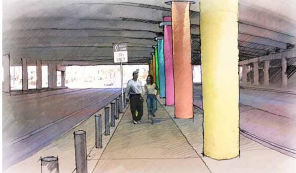
Bollards, lighting and brightly painted elements help make the underpass safer and enliven the space.
