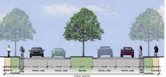
Airline Drive North Proposed Section Scale: 1" = 1'-0"
