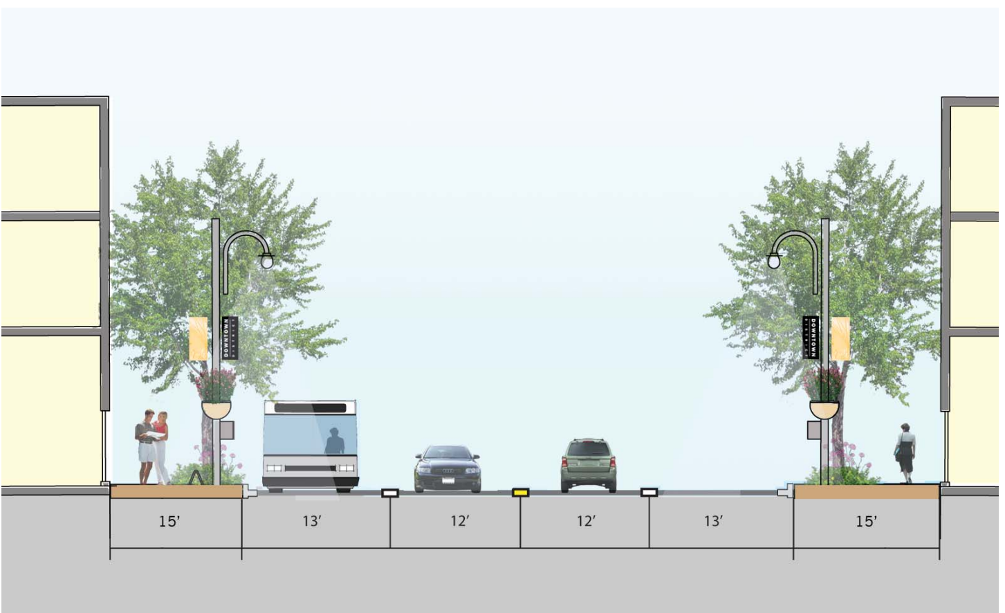
Top Existing conditions on Dowling Street looking north Section Proposed Dowling / Congress Cross Section
