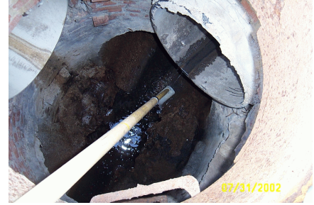
Figure 15. Collecting a sample using telescoping sampling pole.
