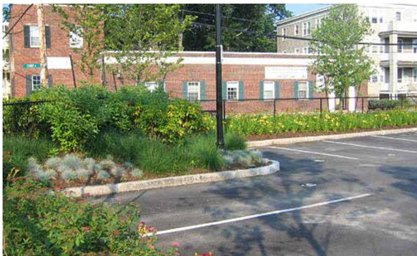
A planting buffer of 10 feet is placed around parking.
