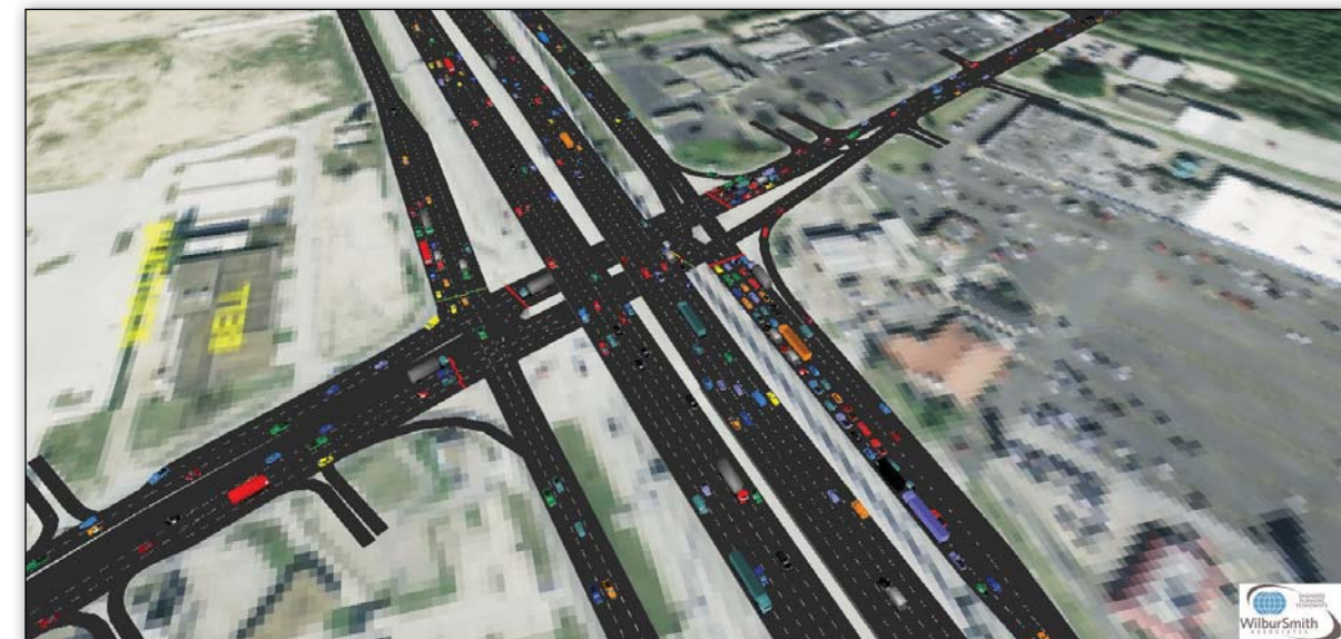
Figure 2.10: VISSIM Model - Screen Capture from Existing PM Peak Simulation - Intersection of FM 2920 and IH 45
