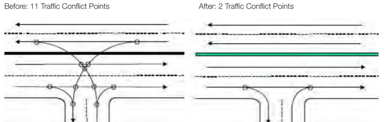
Median U-turns can be implemented along a corridor with medium to high speed four-lane divided highways. Desirable minimum median widths between 40 and 60 ft are typically needed to accommodate large trucks so that they do not encroach on curbs or shoulders. Intersections with narrower medians need bulb-outs or loons at U-turn crossovers. According to the FHWA, a median
