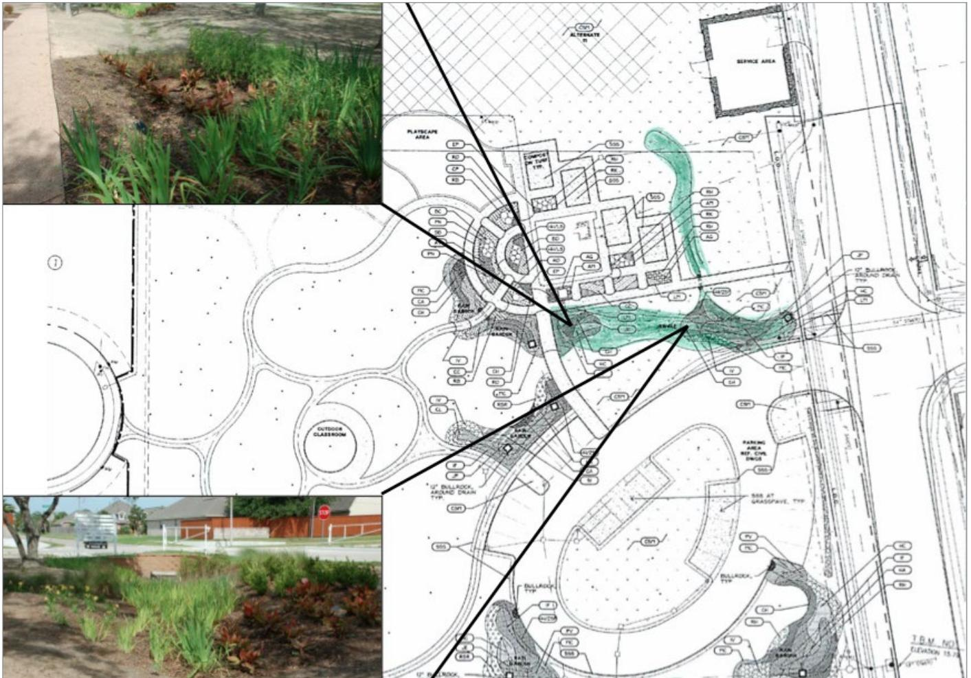
Swales are gently sloping depressions planted with dense vegetation or grass and treat storm water runoff from impervious (solid) surfaces. As the runoff flows along the length of the swale, the vegetation slows and filters the water and allows it to soak into the soil.
