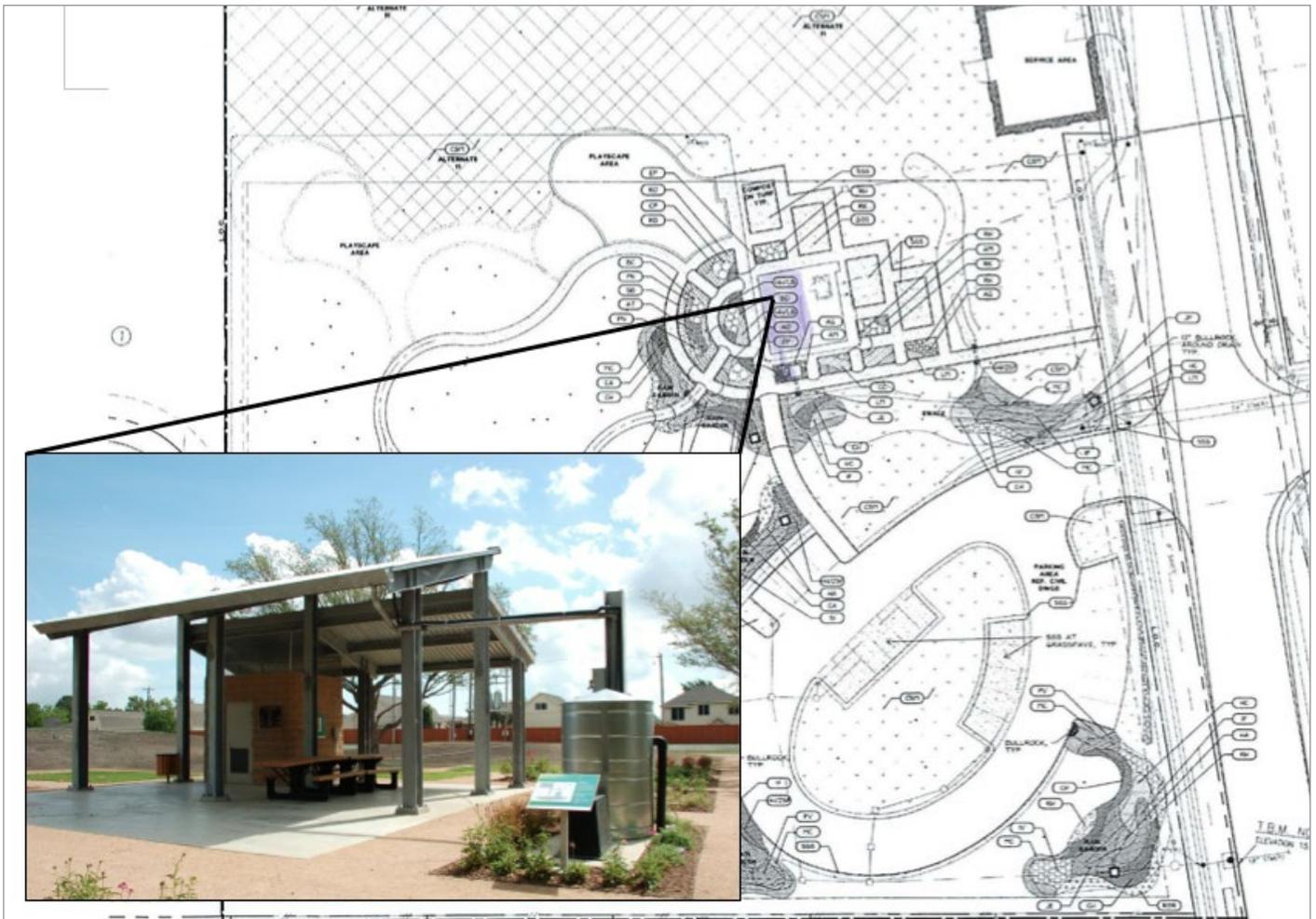
Rainwater harvesting (RWH) is a system that captures, diverts and stores rainwater (storm water) for later use. For storm water control, it retains water to minimize the volume of water entering the storm drain system during a rain event, allows water to be slowly released into the system and recharges groundwater. A RWH system reduces the demand on municipal water supplies while it supplies a better, untreated water source for plants.
