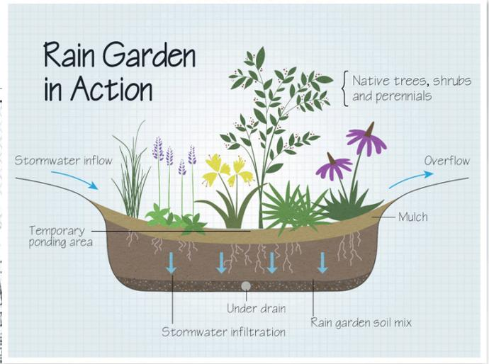
A rain garden is a sunken, generally flat-bottomed garden bed that collects and treats storm water runoff from impervious (solid) surfaces.
