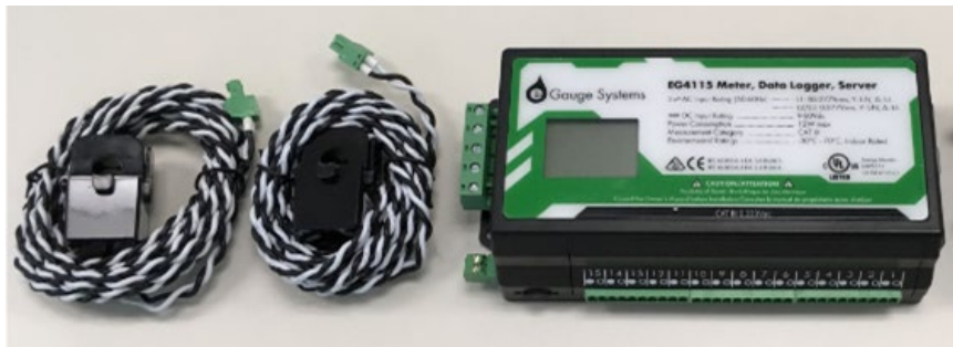
Internet connected energy meter/datalogger
