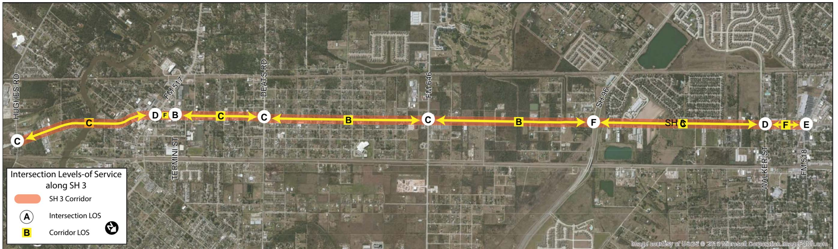
Figure 5-18: SH 3 - LOS for signalized intersections and segments
