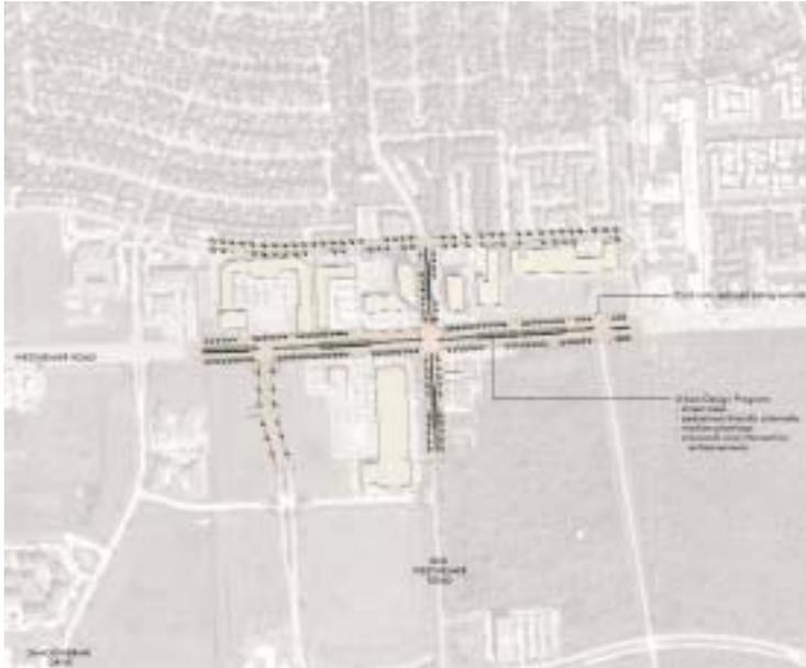
Phase One improvements would start with the Urban Design Program of streetscape improvements along Westheimer, as well as prominent roadways that feed into it. Improvements in this phase would include a consolidation of curb cuts to help streamline traffic movement and direct traffic into existing developments.
