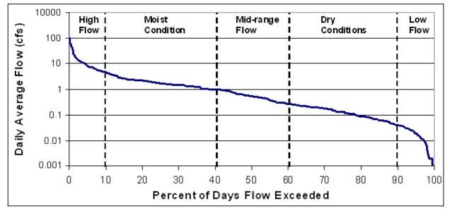
Figure E.1. Example flow duration curve. Vertical axis is flow rate and horizontal axis is percent exceedence. Curve shows percentage of time during a year, on average, a stream exhibits different flow conditions from very high flows during floods to low flow during summer or in long periods of time between rainfall events.
