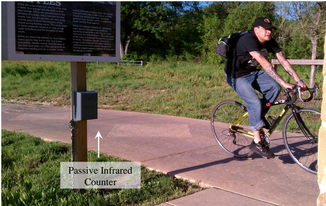
Figure 1-3. Different Types of Infrared Counters for Non-Motorized Traffic.
