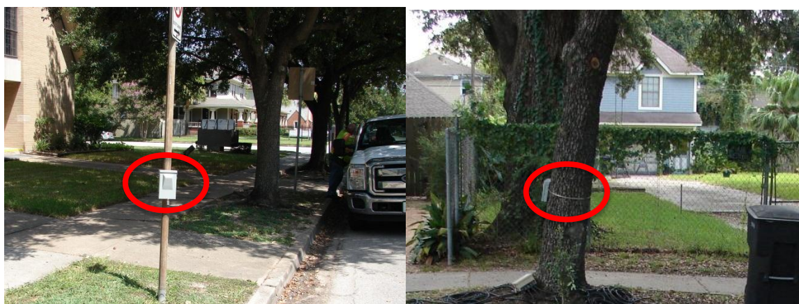
Figure 0-1. Examples of Pedestrian Counter Strapped to No Parking Sign and Tree
