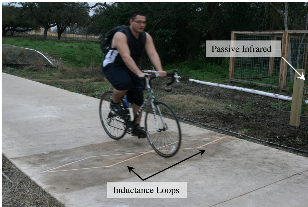
Figure 1-2. Example of Passive Infrared Sensor Combined with Inductance Loop Detectors.
