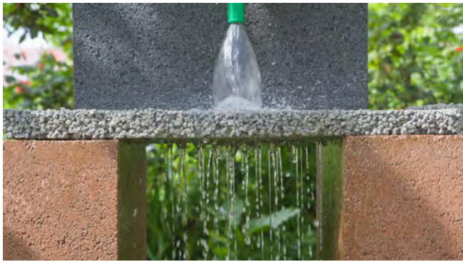
Porous asphalt. Source: waternow.org
