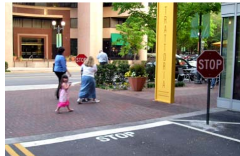
Driveway from parking garage, Arlington VA. Note the double stop signs, one at the sidewalk and one at the street.
