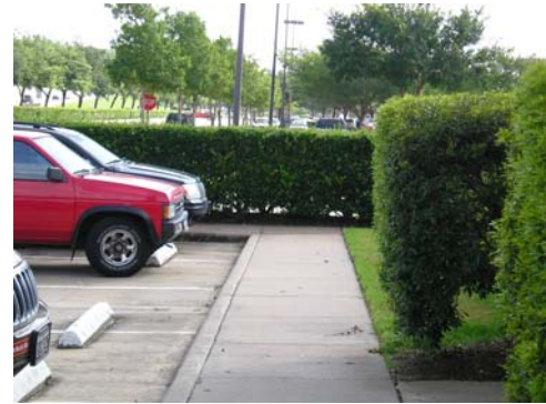
Continuous hedges prevent easy sidewalk access, and pedestrians will often attempt to create and squeeze through small gaps.
