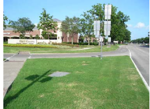
This crosswalk (far left) is so far into the turning lane that motorists will be speeding up before encountering pedestrians.
