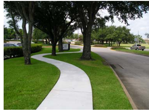
This sidewalk takes an indirect route to its destination and thus adds travel time.
