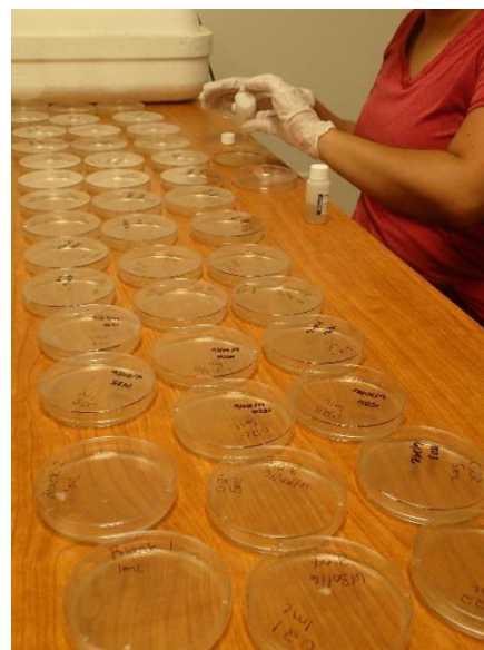
Figure 43. Plating Canal C-147 samples using Coliscan Easygel methodology
