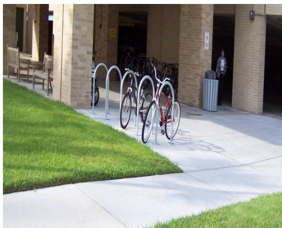
U-type racks like these can be installed singly or in arrays of any number. They provide easier and more secure attachment of bicycles than other designs. U-type racks are available from numerous manufacturers throughout the country.
