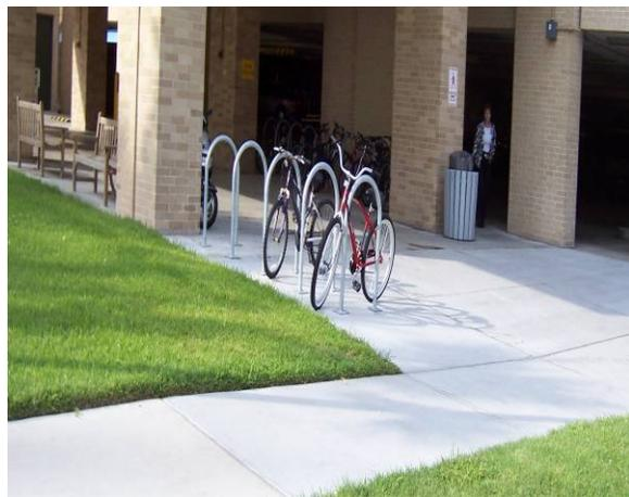
U-type racks like these can be installed singly or in arrays of any number. They provide easier and more secure attachment of bicycles than other designs. U-type racks are available from numerous manufacturers throughout the country.
