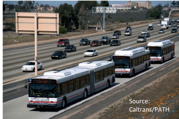
Figure 5 Houston METRO Buses in 1997 During Early Prototype Testing of Platooning Concepts
