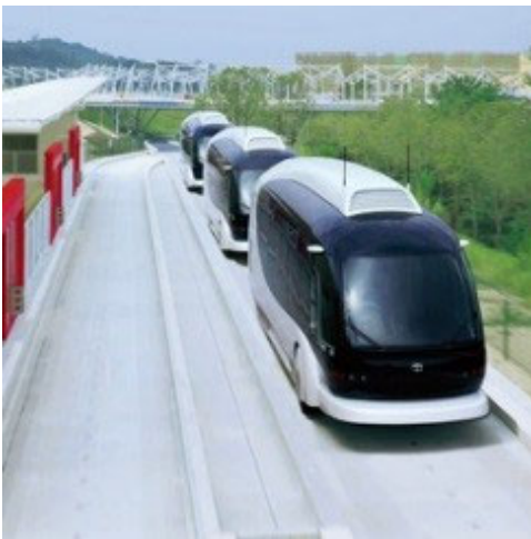
Figure 23 Example of an Off-Line Station for Toyota IMTS Buses Deployed at the 2005 Transportation Expo in Aichi, Japan
