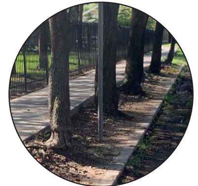
What not to do - rooting soil volume is directly proportional to tree longevity and mature size.
