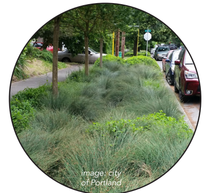
Recommended strategy - large planting beds featuring naturalized plant mixes and ample space for tree rooting. Use of silva cells, structural soils, or suspended pavements should be considered in locations with area constraints.
