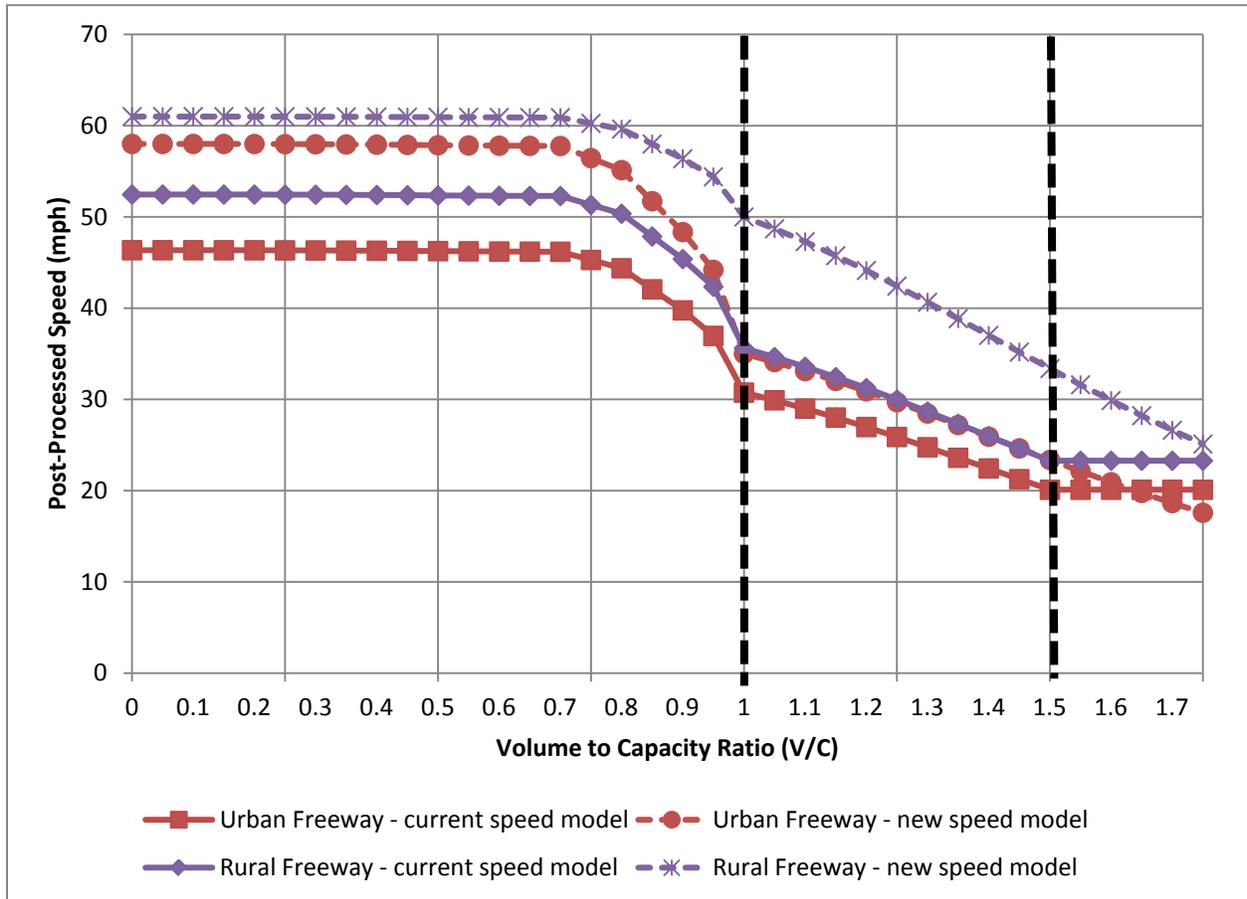
Figure 3. Example Post-Processed Speeds on an Arterial Link
