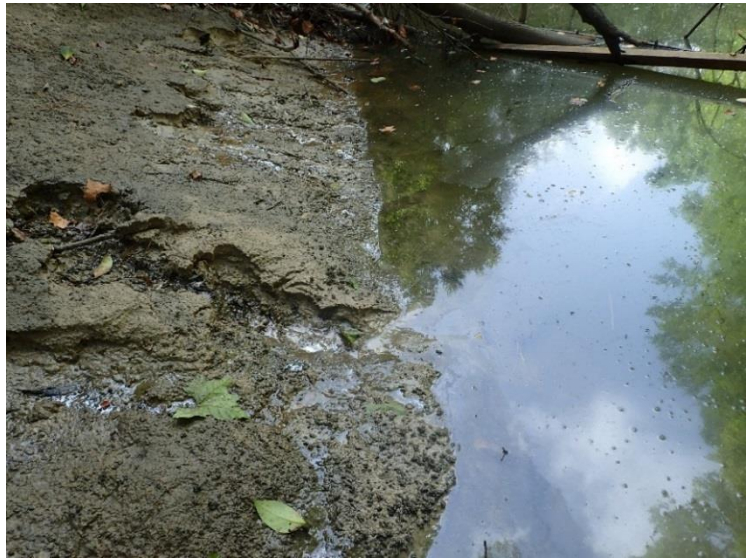
Figure 31. Groundwater discharge and surface sheen at sample 033
