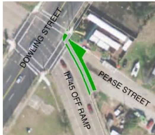
Figure 4.4 Illustration of Project R1-4, Closing of Westbound Pease at Dowling.
