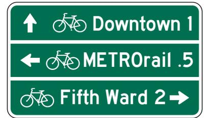
Figure 4.18 MUTCD Destination, Distance and Direction Signs.
