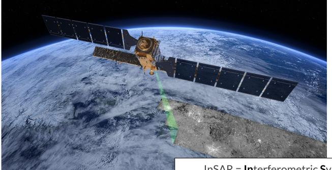
A technique to estimate **mm-scale** displacements
