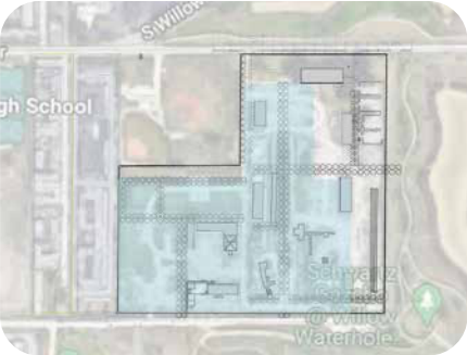
An example of the 75 acre-feet of detention, at 4' deep.
