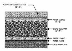
FIGURE 2b POROUS PAVEMENT TYPICAL SECTION
