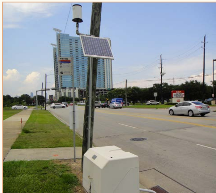
Figure 9. The City of Houston Urban Street Rebuild on Almeda Road automated sampler for the BPA LID BMP preconstruction monitoring project.
