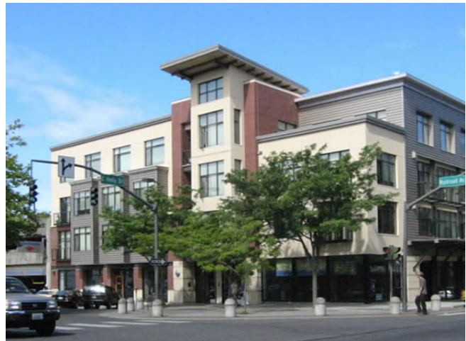
Parapet / flat roofs should have strong cornice detailing, to provide scale and visual interest.
