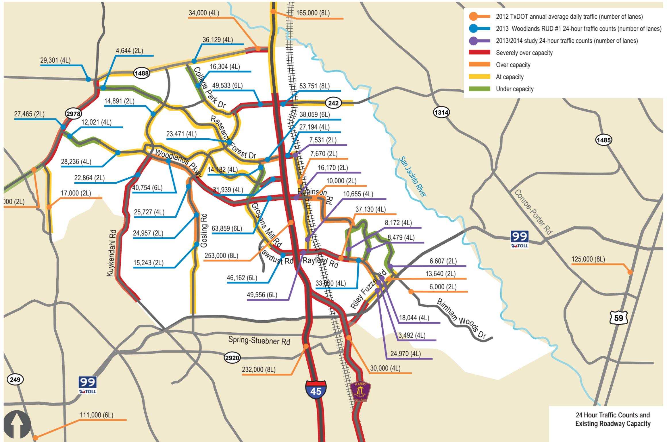
Figure E2: Traffic Counts and Existing Roadway Capacity (Based on roadway capacity analysis, average speed analysis, and delay observed by the helicopter videos.)
