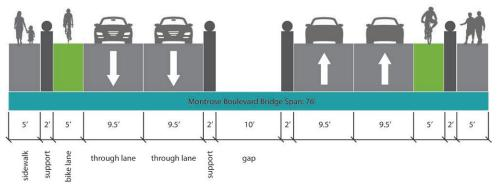
Figure 22. Montrose Boulevard south of Montrose Bridge Existing and Recommended Cross Sections
