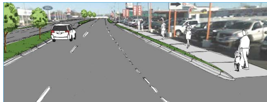
Figure 5.2: Raised median with optional landscaping
