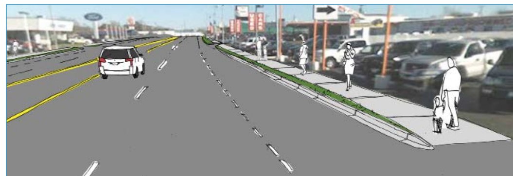
Figure 5.1: Continuous right-turn lane
