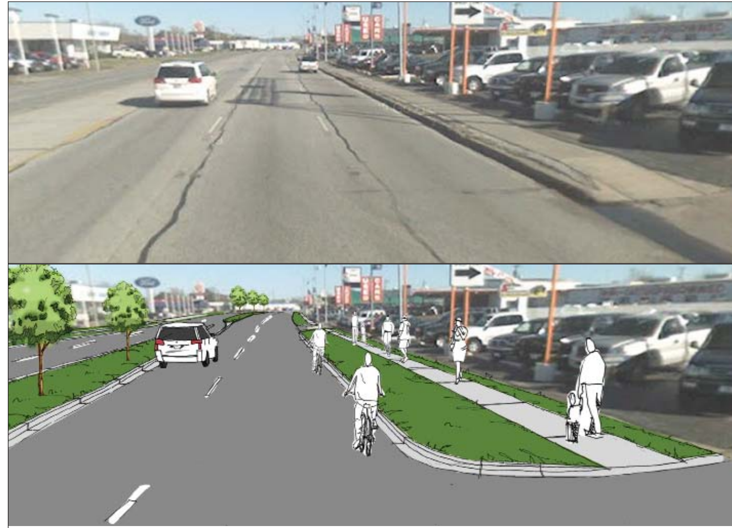
Figure 4.7: Roadway diet; before and after
