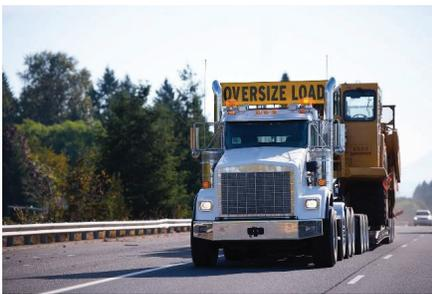
Flooding and the inundation of the pavement structure reduce pavement layer stiffness and have the potential to cause substantial damage to pavement structures. Heavy loads on weakened pavements in the immediate aftermath of a flooding event can lead to sudden failure or severe damage, such as severe cracking, ruts, and potholes. This strategy prohibits oversize/overweight vehicles on inundated pavements or pavement structures until flood water has drained from base layers.
