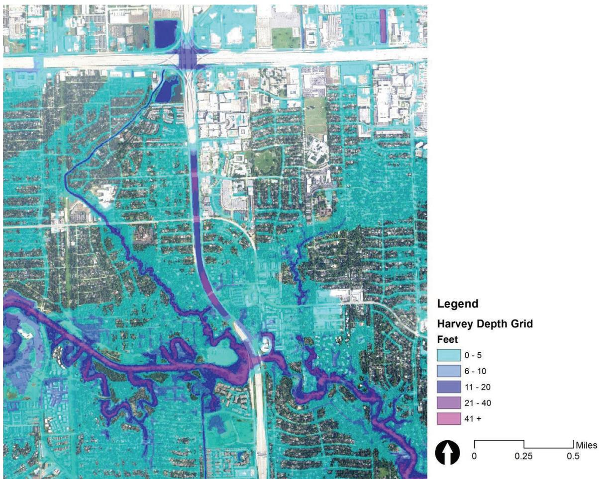
4. **Exposure Depth**- Exposure depth grid is a 5-by-5-meter raster grid representing flood level on top of a structure, such as a roadway or bridge section. The value of exposure depth grid is equal to the difference between roadway/bridge surface elevation, or DSM, and flood WSEL (see Figures 29 and 30). Exposure depth for roadway segments and bridges was measured using the various water depth data mentioned in the previous section.
