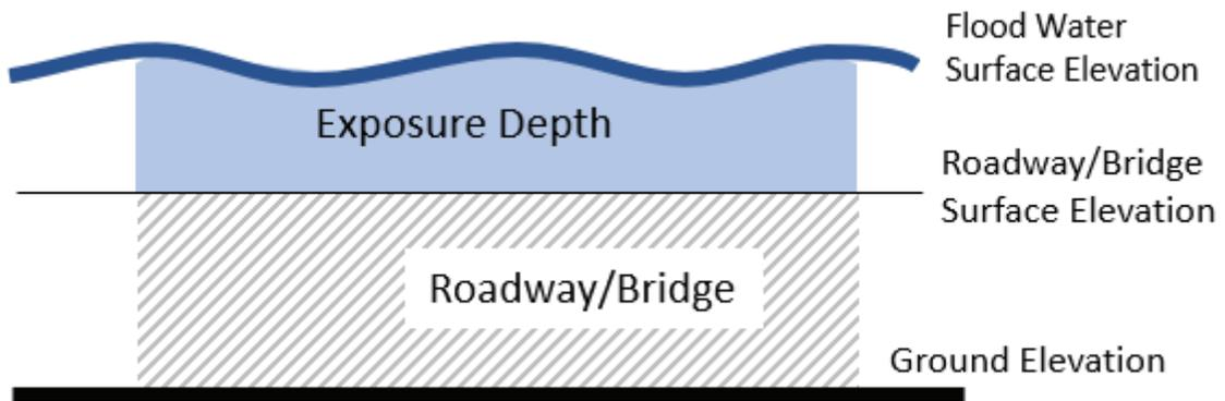
Figure 30 – Exposure Depth Grid
