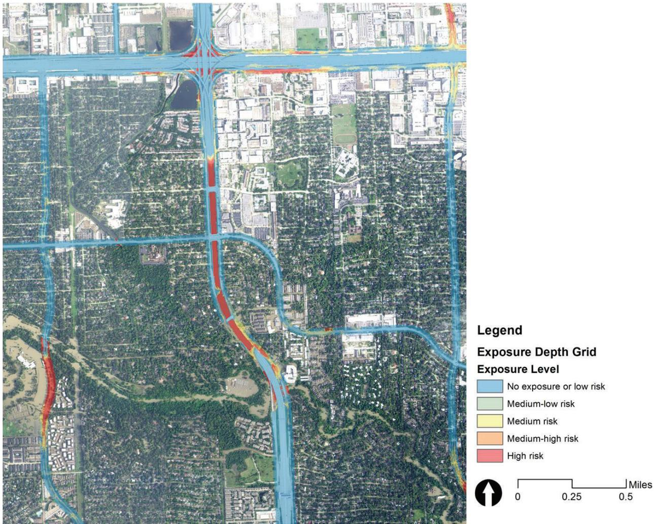
Figure 32 shows the exposure depth grid data for Highway 288 at Holly Hall Street. The model estimates a portion of the highway at this location as high risk for flooding even though it is outside the 500-year flood plain. This estimate is validated by the flooding that occurred on September 22, 2020, because of Tropical Storm Beta.
