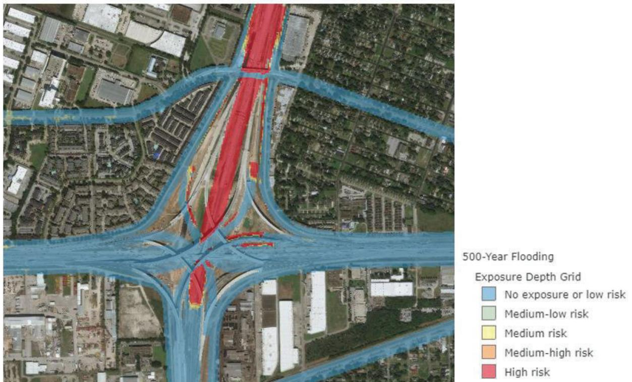
Figure 33, an image from ABC 13, shows the same portion of the Highway 288 flooded as indicated by the modeled high-risk exposure depth grid data. Detailed methodology of the LiDAR data processing and flood modeling are documented in Appendix B on page 124.
