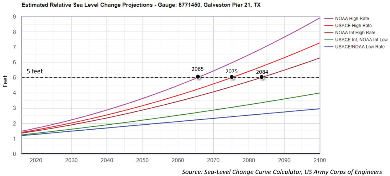
Per the NOAA Sea Level Rise Viewer, the sea level of Galveston Pier 21 area with 'High' scenario will reach 5 feet higher than current Mean Higher High-Water level around 2070 (see Figure 21).
