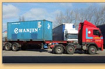
Combination Trucks Carrying Intermodal Shipping Containers Boxes with Specially Designed Corners (Can Be Lifted from Above)
