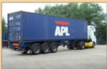
Combination Trucks Carrying Intermodal Shipping Containers Boxes with Specially Designed Corners (Can Be Lifted from Above)
