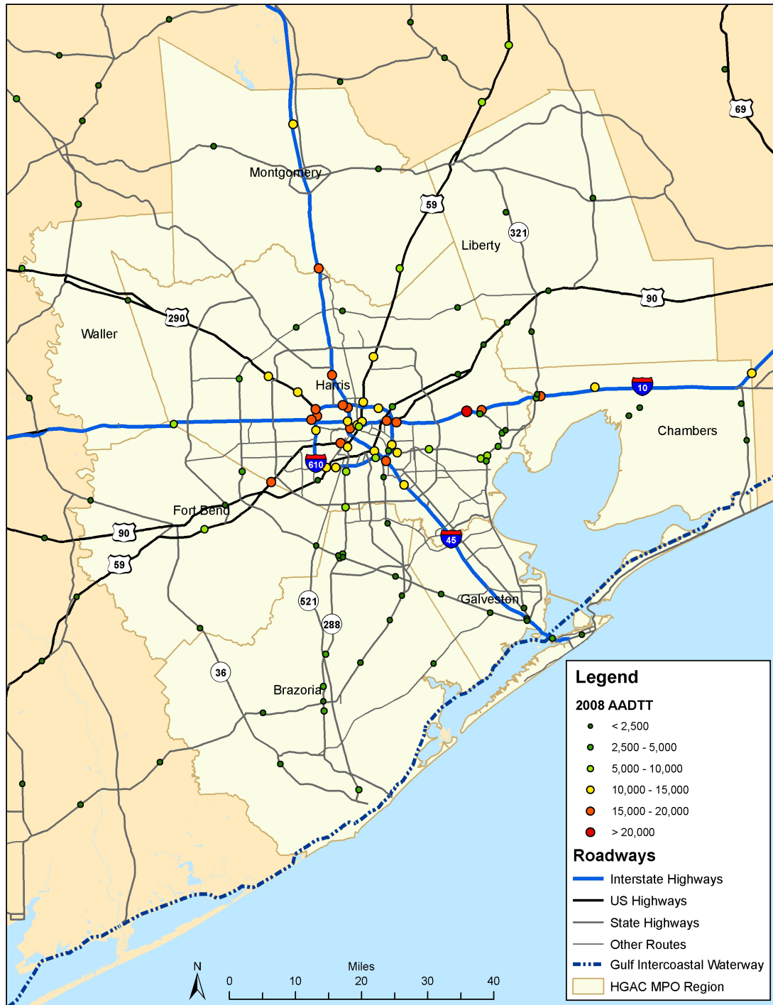
Figure 2.6 Truck Counts at Permanent Count Locations – 2008
