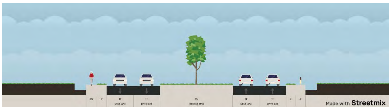
Figure 12: Typical 4-lane roadway cross section of West Bellfort Avenue, east of South Gessner Road
