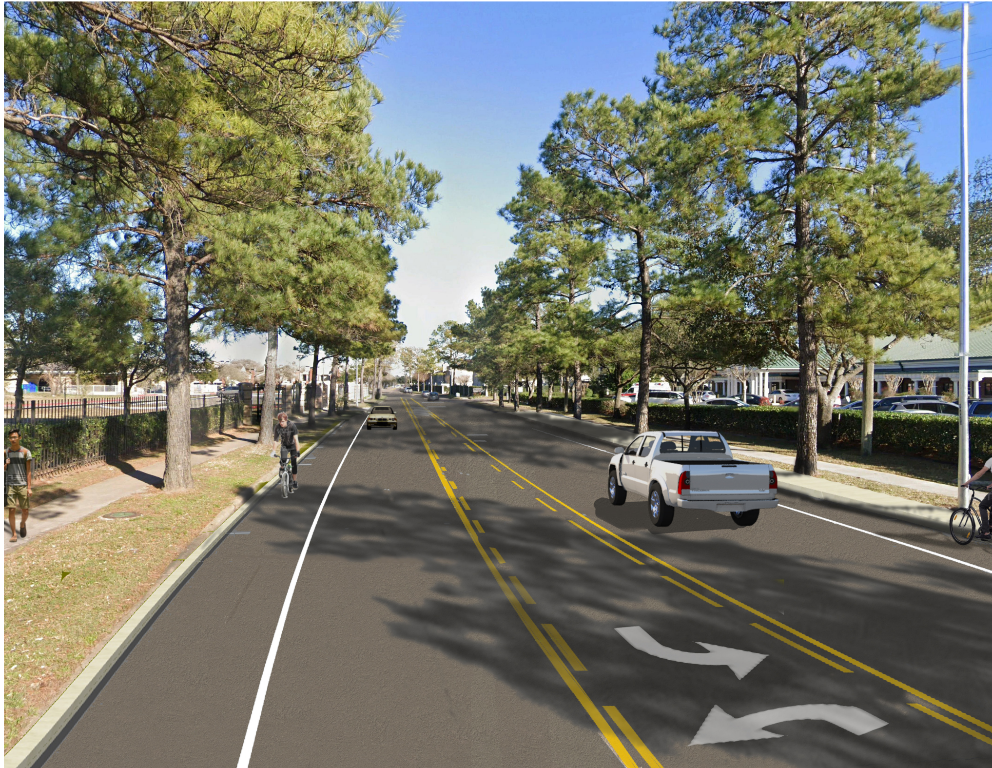
Implementing a road diet on Creekbend Drive would improve active transportation connectivity and improve safety for all users.
