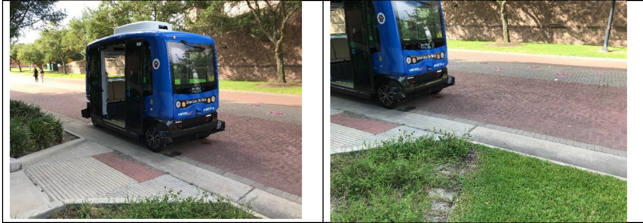
Figure 2-10 Example of a Misaligned Vehicle Stopping Location Due to Vegetation Movement Adjacent to the Programmed Station Stop Affecting the Lidar Sensors
