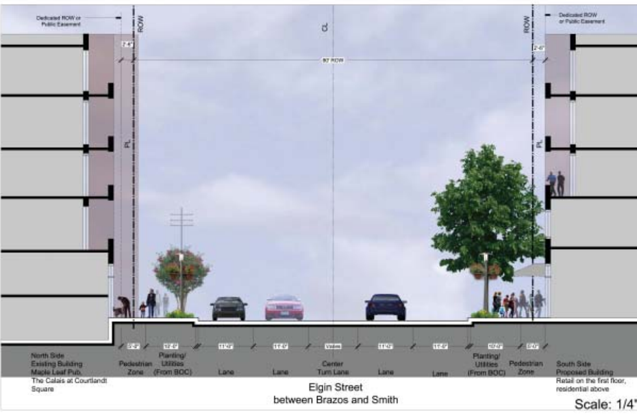
Improvements with Utilities Buried on One Side
