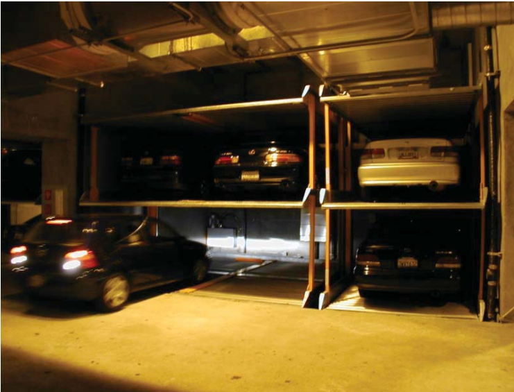
Parking stackers: an example of a strategy to quickly and cost-effectively increase parking capacity to meet demands Photo: Nelson\Nygaard
