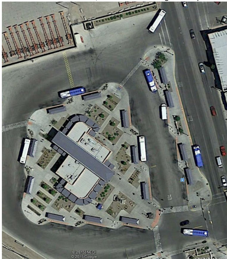
Figure D-3 Off-Line Station Configuration With Individual Vehicle Berths
