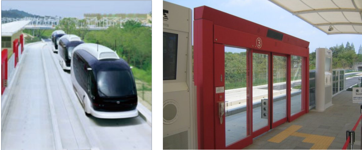
Figure D-2 Off-Line Station With Platform Edge Doors Deployed by Toyota for the Automated Buses at the 2005 Aichi Expo
