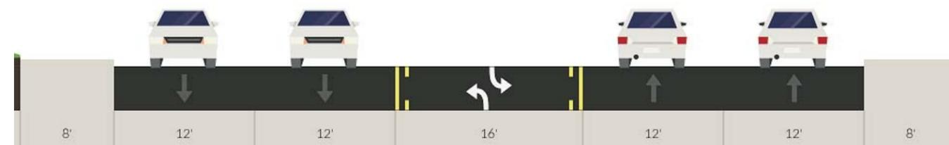
Figure 9 – Existing SH 146 Cross-Section
