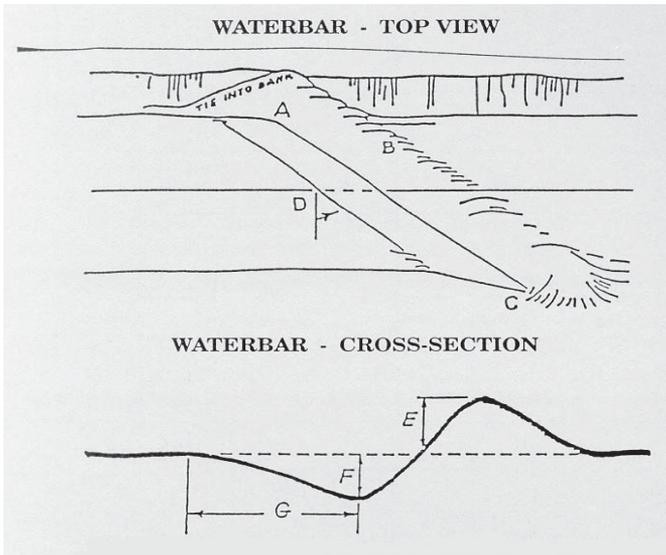
1. Specifications for waterbar construction on forest roads, trails and firebreaks must be site specific and should be adjusted to existing soil and slope conditions.
