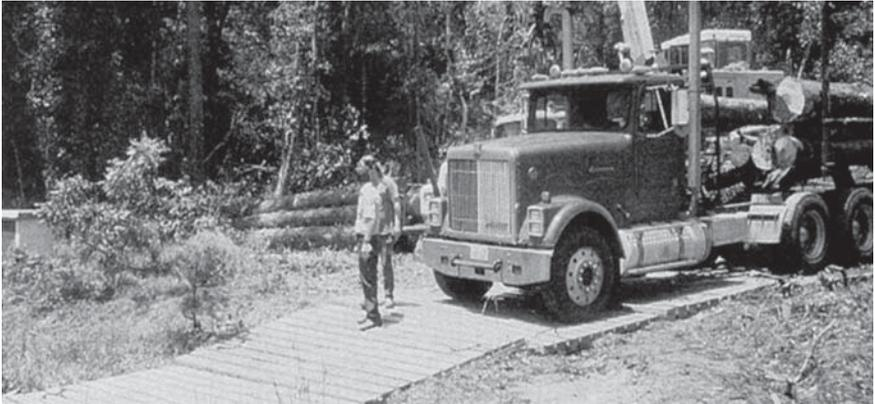
Use board road or wooden mats where needed to minimize rutting.
