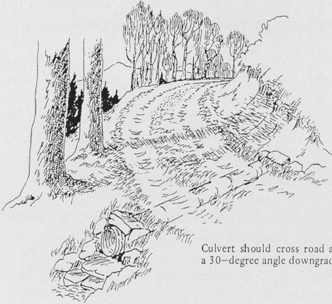
Culvert should cross road at about a 30-degree angle downgrade.
