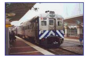
Figure 3-1 – Trinity Railway Express operates diesel locomotive-hauled coaches.
