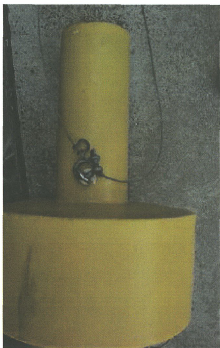
Photo 11 - D-rings shackled directly to the "eye" of the buoy.
