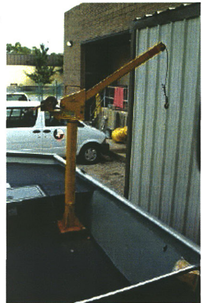
Photo 7 - Crane mounted on deck of boat.
