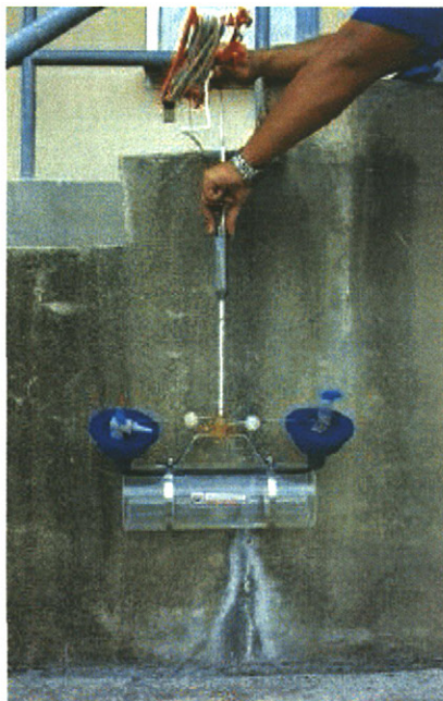
Photo 10 - Van Dorn bottle used to collect stratified water samples.
