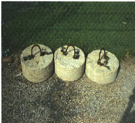
Photo 4 - Concrete weights showing chain and locking shackles.
