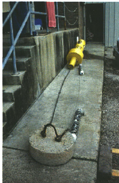
Photo 8 - Buoy and weight assembly with attached sondes.
