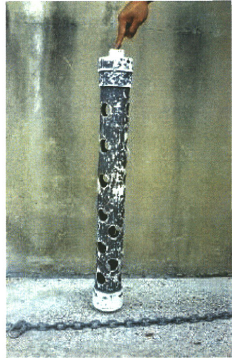
Photo 9 - Protective PVC cover for sonde deployment.
