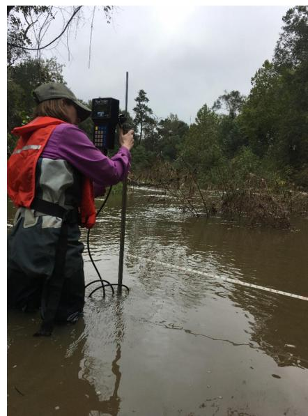
Image: Kendall Guidroz conducts flow monitoring at a Clean Rivers Program location.
