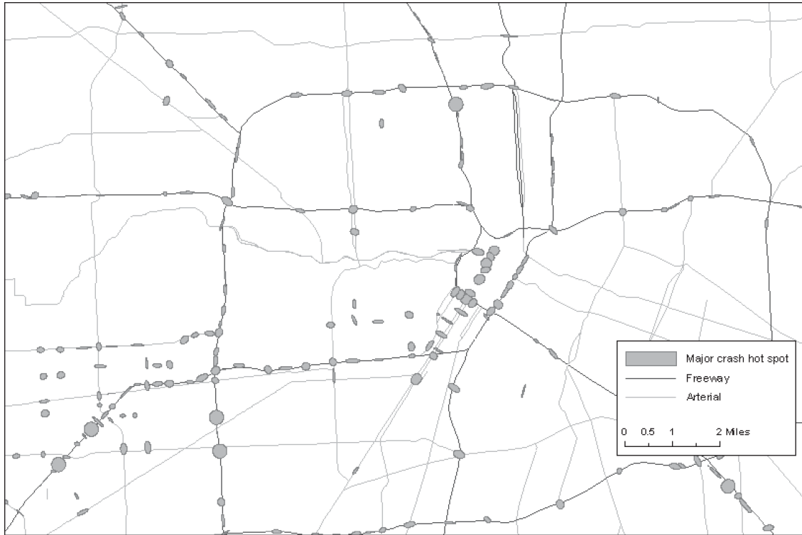
FIGURE 3 Central Houston major crash hot spots—locations of hot spots with 78 or more crashes, 1999 to 2001.
