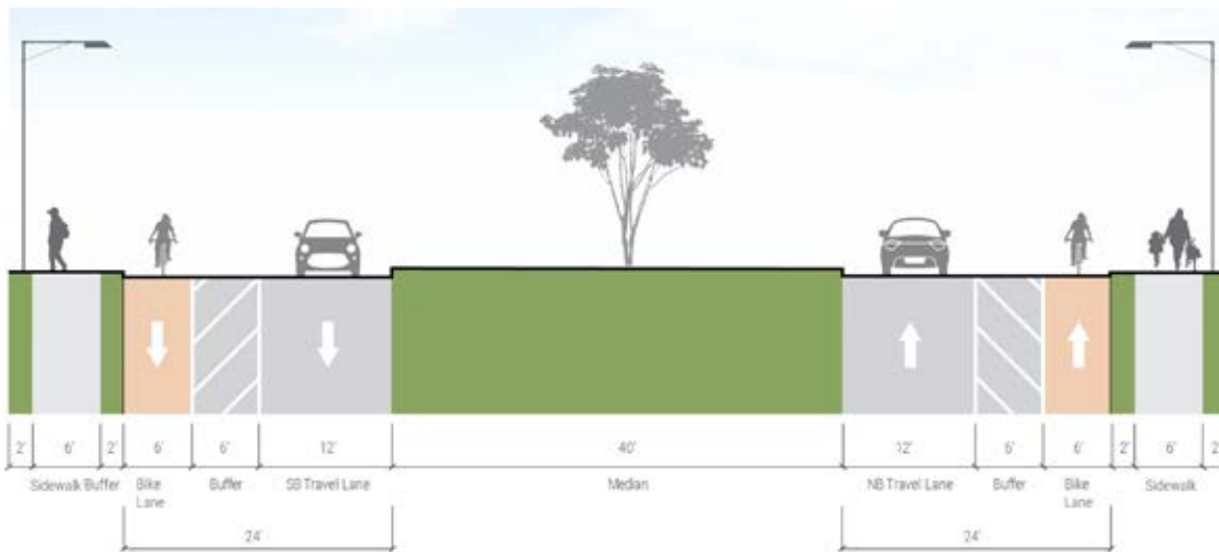
Hirsch / Broyles / Altoona / Waco Street, from I-610 North Loop to I-10 East Freeway, after reallocation.
