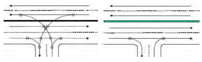
Median U-turns can be implemented along a corridor with medium to high speed four-lane divided highways. Desirable minimum median widths between 40 and 60 ft are typically needed to accommodate large trucks so that they do not encroach on curbs or shoulders. Intersections with narrower medians need bulb-outs or loons at U-turn crossovers. According to the FHWA, a median
