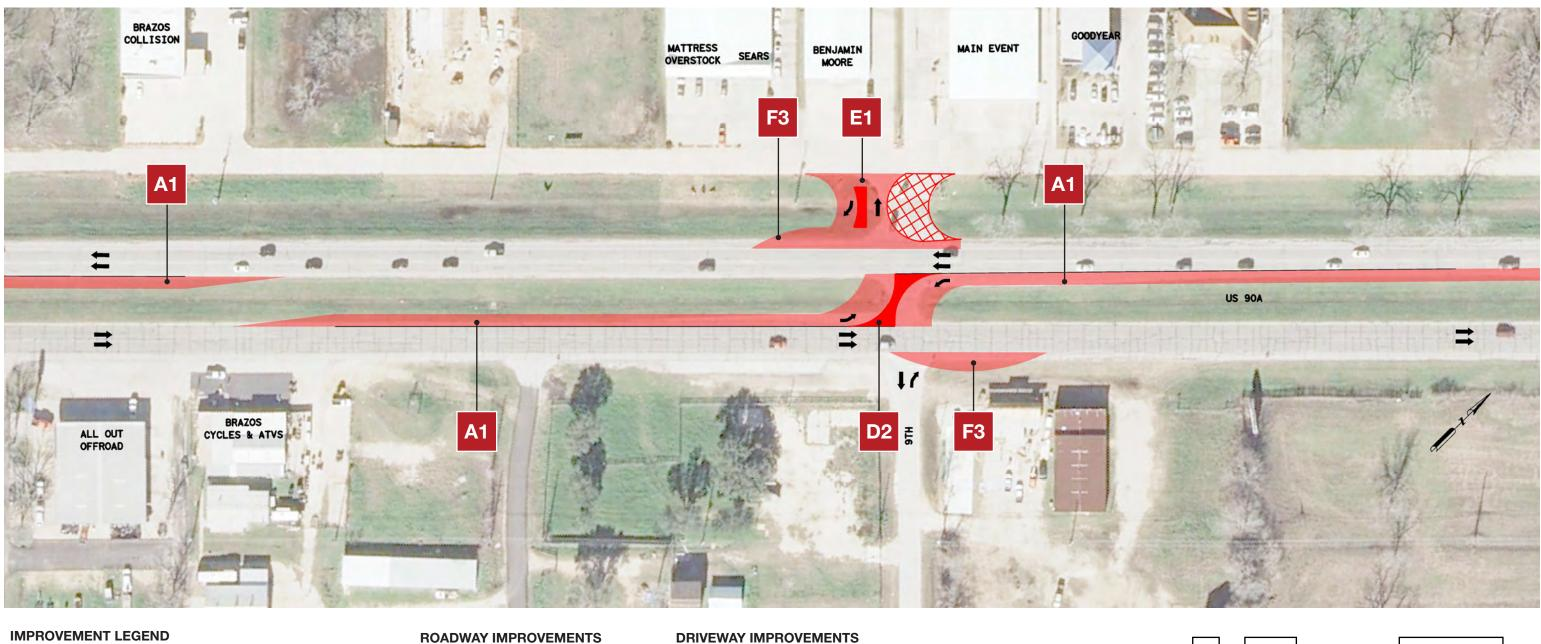
K Remove Pavement New Pavement — Pavement Striping Improvement by County Improvement by TxDOT Improvement by City
