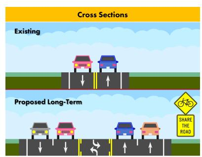
Figure ES-5: Example Roadway Recommendations Cross Sections
